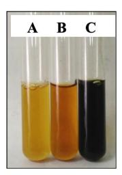
Figure-1: Sample tubes containing Ferric chloride solution (A), *P. marsupium* bark extract (B) and FeNPs solution (C)
