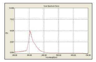
Figure-2: UV-Vis absorption peak of biosynthesized FeNPs.
