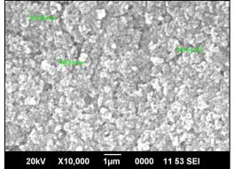
Figure-3: SEM image of biosynthesized FeNPs from *P. marsupium* bark extract
