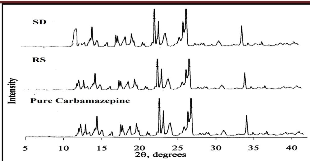
Figure-3 XRD spectra of different samples of Carbamazepine
