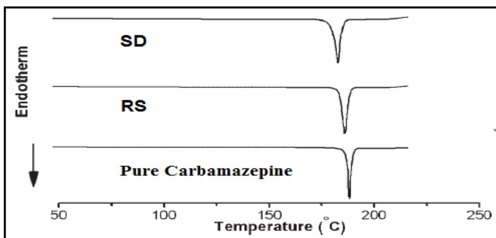
**Figure-1 DSC spectra of different samples of Carbamazepine**
