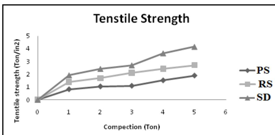
Figure 5– Tensile strength of P.S-pure Sample, R.S-Recrystallized sample, S.M-spray dried microparticle
