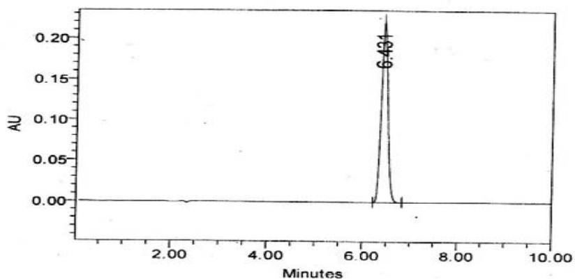
Fig 2: A typical chromatogram For Nicorandil
