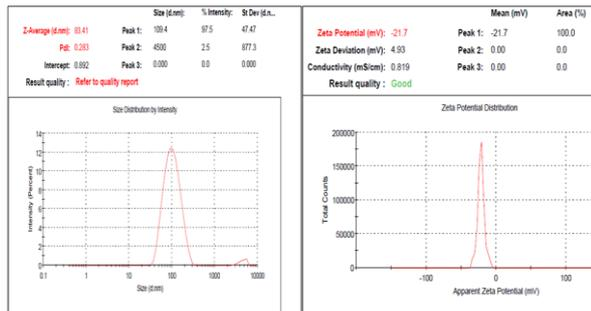
Figure 3: Characterization of SNPs by a) DLS b) Zeta potential
