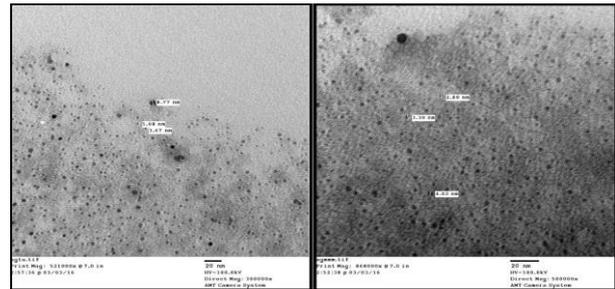
Figure 2: TEM of SNPs at resolution a) 300000x b) 500000x
