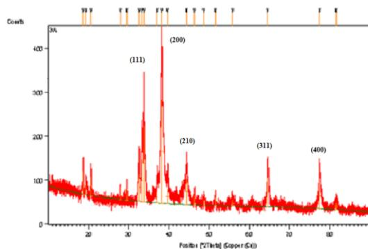
Figure 5: X-ray diffraction pattern of SNPs
