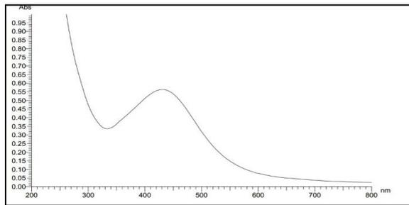
Figure 1: UV-Visible absorption spectra of colloidal solution synthesized SNPs
