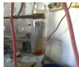
Fig.2, Soxhlet Appratus For Extraction
